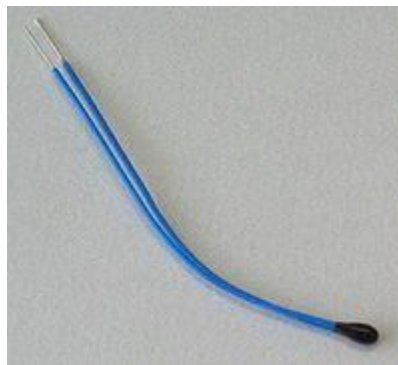
NTC (negative temperature coefficient)
