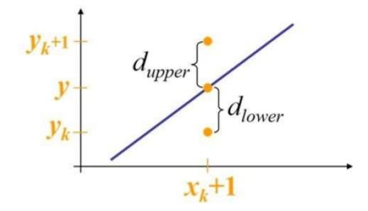
From the above illustration, the y coordinate on the mathematical line at xk+1xk+1 is -Y = m(XkXk+1) + b
