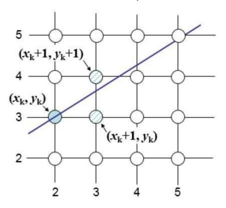
At sample position Xk+1,Xk+1, the vertical separations from the mathematical line are labelled as dupperdupper and dlowerdlower.
