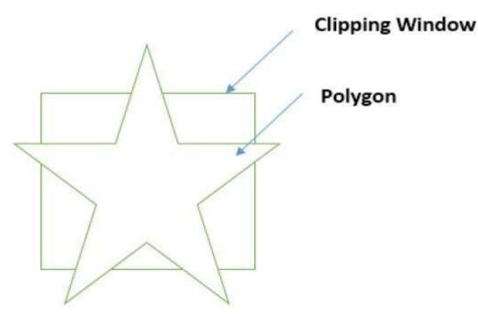
While processing an edge of a polygon with clipping window, an intersection point is found if edge is not completely inside clipping window and the a partial edge from the intersection point to the outside edge is clipped. The following figures show left, right, top and bottom edge clippings –
