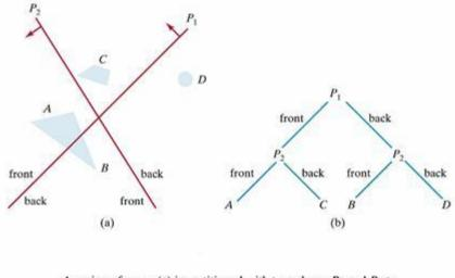
A region of space (a) is partitioned with two planes  $P_1$  and  $P_2$  to form the BSP tree representation shown in (b).
