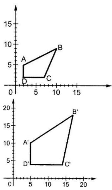
If we provide values less than 1 to the scaling factor S, then we can reduce the size of the object. If we provide values greater than 1, then we can increase the size of the object.
