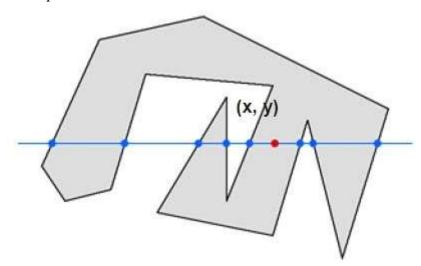
From the above figure, we can see that from the point (x,y), the number of interactions point on the left side is 5 and on the right side is 3. From both ends, the number of interaction points is odd, so the point is considered within the object.
