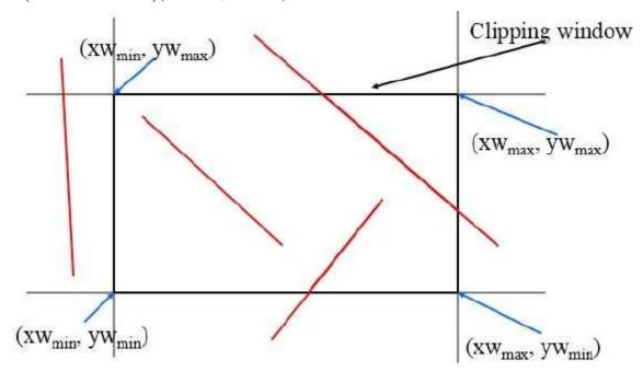
We will use 4-bits to divide the entire region. These 4 bits represent the Top, Bottom, Right, and Left of the region as shown in the following figure. Here, the **TOP** and **LEFT** bit is set to 1 because it is the **TOP-LEFT** corner.
