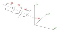
In the above figure, S1, S2, S3 are the surfaces and (x,y) is the view-plane position. The surface which is closest to the projection plane is called the visible surface.
