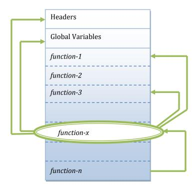
Figure 3.2: A function (in C) is not well-encapsulated
