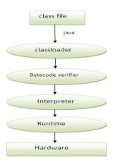
**Class loader:** is the subsystem of JVM that is used to load class files. **Bytecode Verifier:** checks the code fragments for illegal code that can violate access right to objects.
