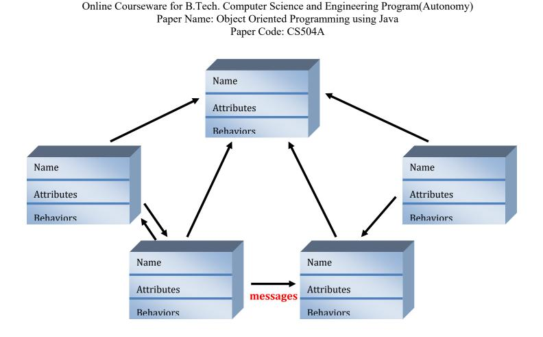
Figure 3.3.1: An object-oriented program consists of many well-encapsulated objects and interacting with each other by sending messages
