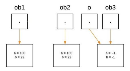
• Now as we can see, equalTo method is called on 'ob1', and 'o' is referring to 'ob3'. Since values of 'a' and 'b' are not same for both the references, so if(condition) is false, so else block will execute and false will be return.
