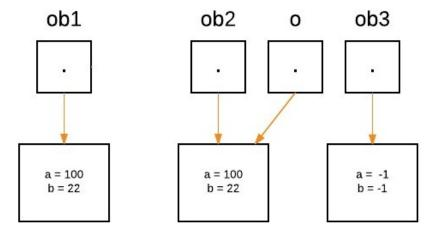
• Now as we can see, equalTo method is called on 'ob1', and 'o' is referring to 'ob2'. Since values of 'a' and 'b' are same for both the references, so if(condition) is true, so boolean true will be return.
