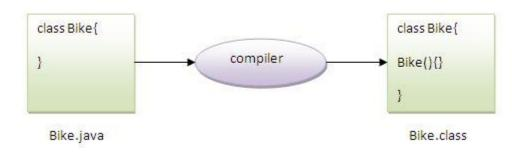
**Note** –Default constructor is used to provide the default values to the object like 0, null etc. depending on the type.
