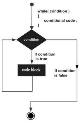
Here, key point of the while loop is that the loop might not ever run. When the expression is tested and the result is false, the loop body will be skipped and the first statement after the while loop will be executed.
