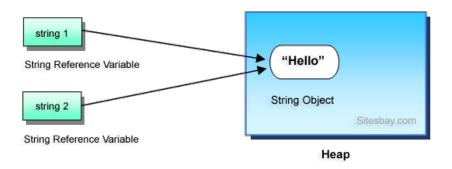
Java String contains an immutable sequence of Unicode characters. Java String is different from string in C or C++, where (in C or C++) string is simply an array of char. String class is encapsulated under java.lang package.
