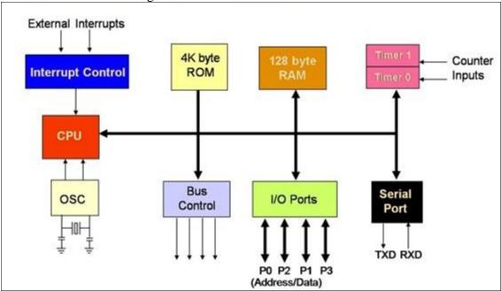
Figure 4.1: Block Diagram of 8051 Microcontroller
