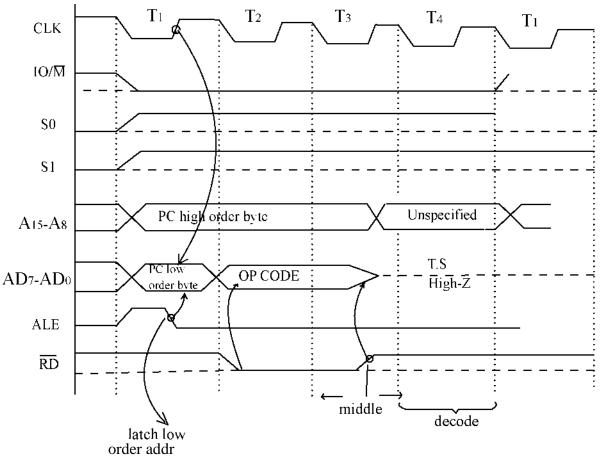
Fig.2.2 Timing Diagram During 4-state OpCode Fetch Machine Cycle
