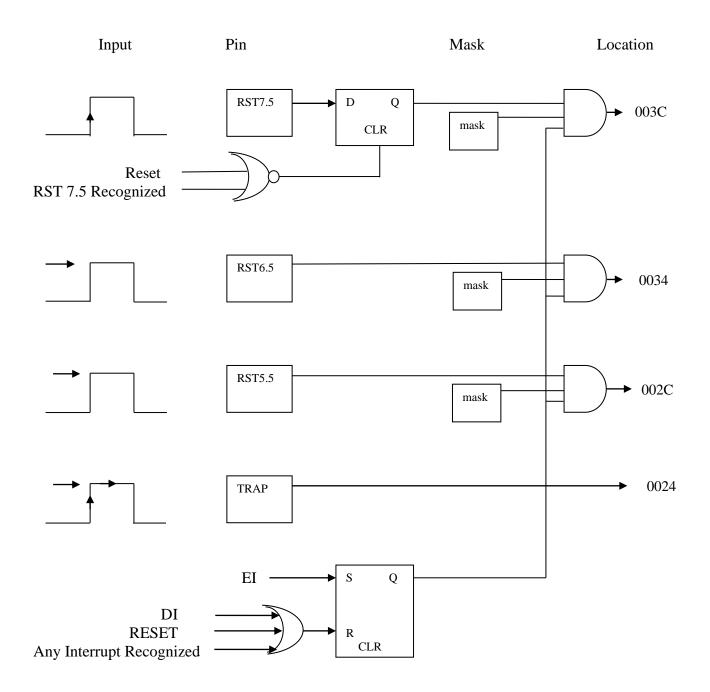
Figure 1.2: Hardware for 8085 Vectored Interrupts
