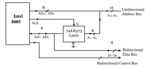
Fig.1.5b: De-multiplexing of AD bus to Generate System Bus
