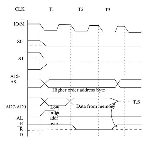
Fig. 2.3 Timing Diagram During Memory Read Machine Cycle
