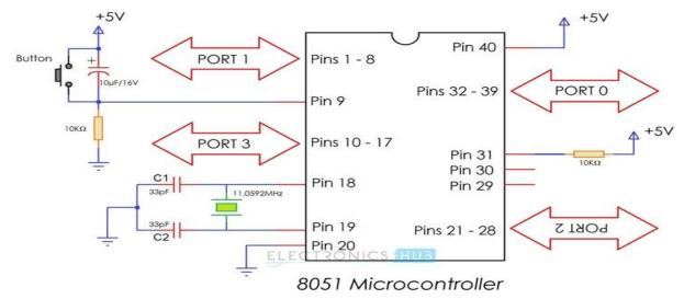
Figure 4.5: 8051 Microcontroller Basic Circuit
