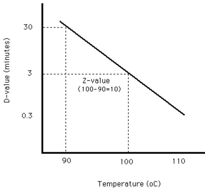
Reactions that have small Z values are highly temperature dependent, whereas those with large Z values require larger changes in temperature to reduce the time. A Z value of 10°C is typical for a spore forming bacterium. Heat induced chemical changes have much larger Z values than microorganisms, as shown below.
