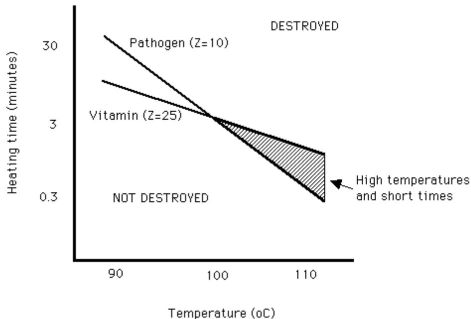
Alkaline phosphatase is a naturally-occurring enzyme in raw milk which has a similar Z value to heat-resistant pathogens. Since the direct estimation of pathogen numbers by microbial methods is expensive and time consuming, a simple test for phosphatase activity is routinely used. If activity is found, it is assumed that either the heat treatment was inadequate or that unpasteurized milk has contaminated the pasteurized product.
