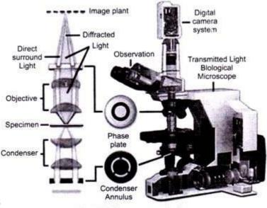
Fig. 6.4 Phase-contrast microscope
