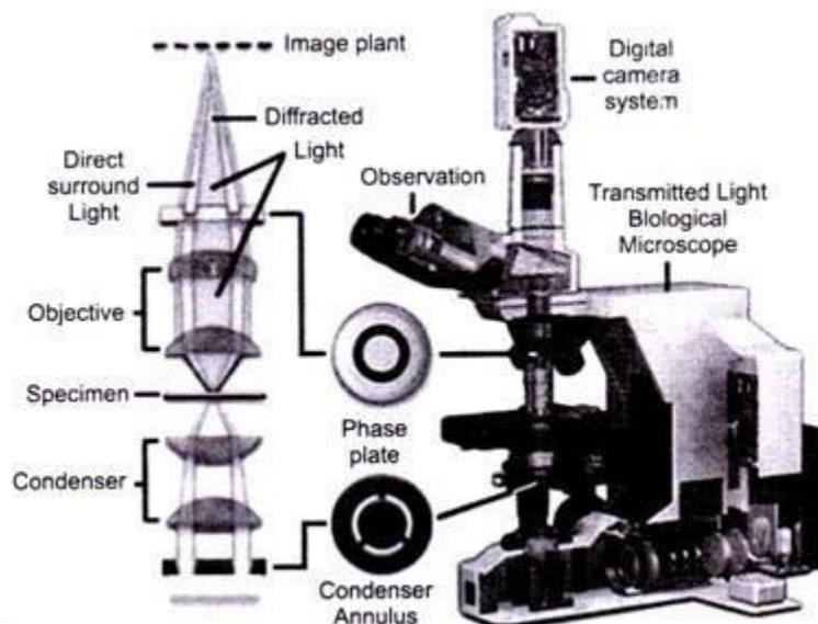
Fig. 6.4 Phase-contrast microscope
