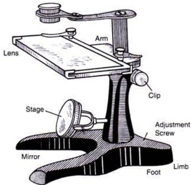
Fig. 6.1 Simple/dissecting microscope
