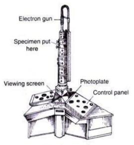
Fig. 6.3 An electron microscope
