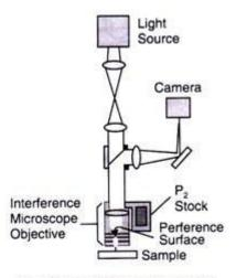
Fig. 6.5 Interference microscope
