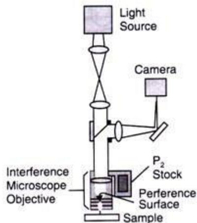
**Fig. 6.5** Interference microscope
