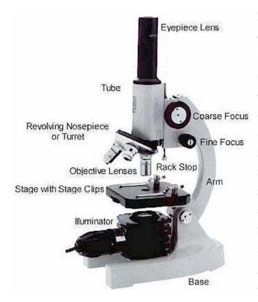
Compound Microscope and its different parts
