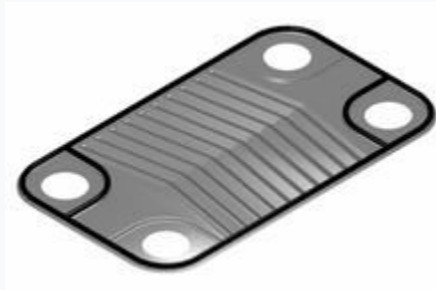
Conceptual diagram of a plate and frame heat exchanger.
