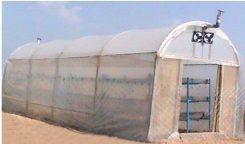
Figure 2: A basic design of the tunnel solar dryer
