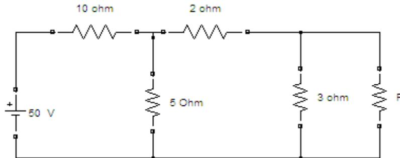
8.c) Determine current through the resistance R using Millman's theorem.
