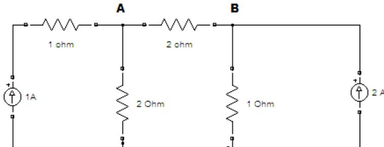
6. State Superposition Theorem. Using this theorem calculate the current through the R of the circuit shown in the figure below.
