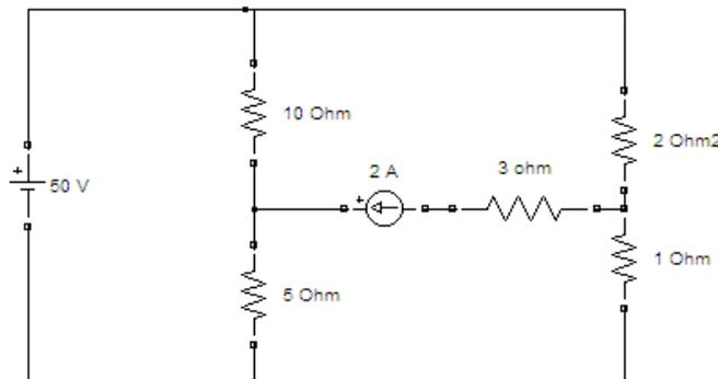
7. b) State Superposition Theorem. Using this theorem calculate the current through the R of the circuit shown in the figure below..
