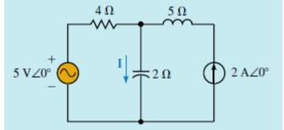
10.a) Derive the expression for resonant frequency for the parallel circuit 5 CO3 shown in figure.
