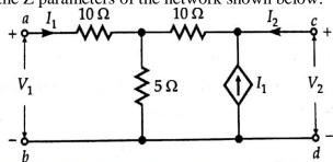
8.c) Find Y parameters for the network. Determine whether the network is 5 CO4 symmetrical and reciprocal.
