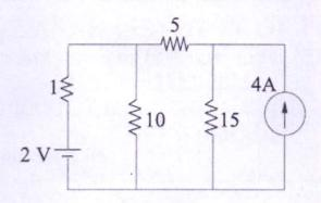
3. a) Using KCL find all the branch currents following the figure below:
