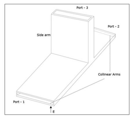
The following figure shows the connection made by the sidearm to the bidirectional waveguide to form the parallel port.
