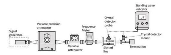
Figure: Microwave Test bench
