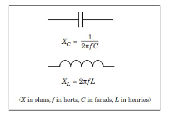
Figure 1  $\cdot$  The simplest frequency-dependent behaviors are capacitive and inductive reactance.
