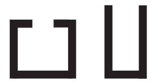
Figure 4: Two possible shapes of open-loop resonator.
