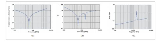
Figure  $2 \cdot$  Frequency-dependent behavior of a 100 pF chip capacitor: (a) reactance, (b) Q, and (c) effective series resistance (ESR).
