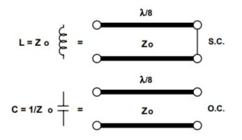
The  $\lambda/8$  transmission line sections are called commensurate lines, since they are all the same length in a given filter. Kuroda's idea is use the  $\lambda/8$  line of appropriate Zo to transform awkward or unrealizable elements to those with more tractable values and geometry. As an example, the series inductive stub in the diagram here can be replaced by a shunt capacitive stub on the other end of the  $\lambda/8$  line, with different values of characteristic impedance determined by
