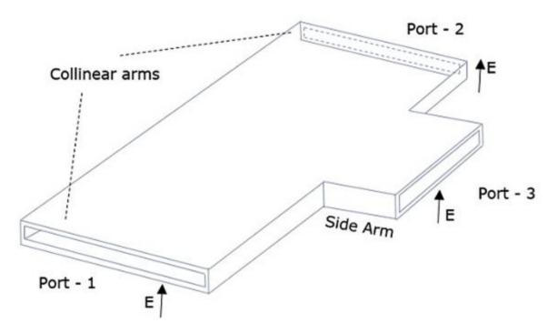
The following figure shows the connection made by the sidearm to the bidirectional waveguide to form the serial port.
