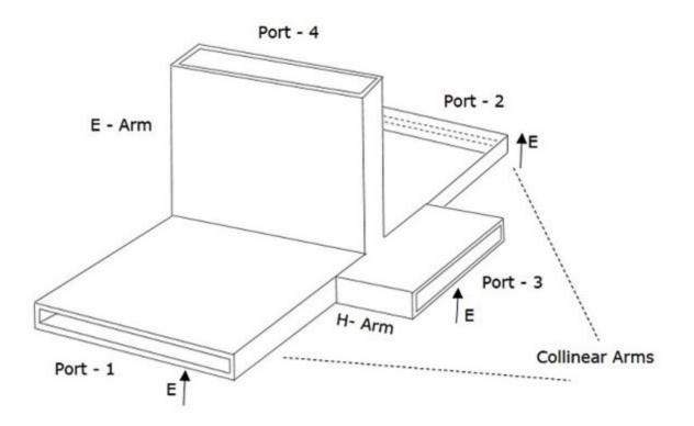
The following figure shows the connection made by the side arms to the bidirectional waveguide to form both parallel and serial ports.
