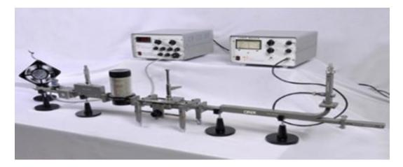
Figure: Microwave Test bench(Practical Example)
