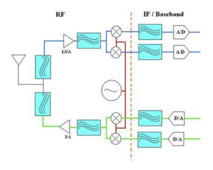
**Figure:** Filters are needed extensively inside and outside the RF transceivers. Better performance of the external discretes allows internal IF and base-band filters to share a common path among different protocols and bands.[2]
