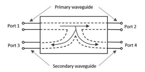
Directional coupler is used to couple the Microwave power which may be unidirectional or bi-directional.
