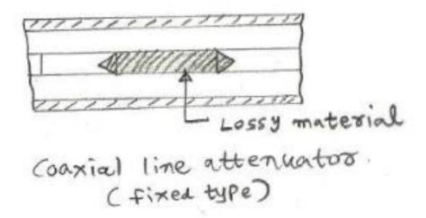
This figure depicts coaxial line based fixed type of attenuator. Here resistive film is fixed at the centre conductor which absorb the power and as a result of power loss and hence microwave signal gets attenuated. This is referred as coaxial line attenuator.
