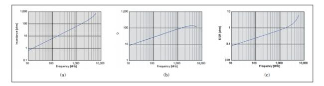
Figure  $3 \cdot$  Frequency-dependent behavior of a 10 nH chip inductor: (a) impedance, (b) Q, and (c) effective series resistance (ESR).
