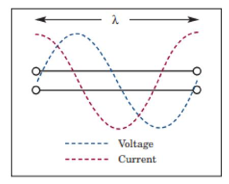
Figure 4  $\cdot$  Voltage and current on a one-wavelength long transmission line.
