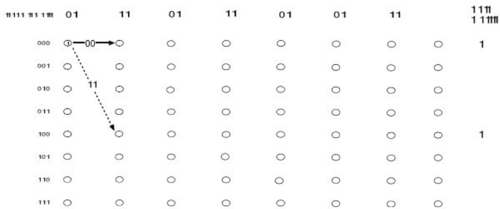
Viterbi Decoding, Step 1
