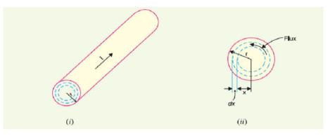
Fig 1.2: Internal flux linkage in a cylindrical conductor
