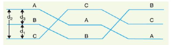
Fig 1.9: Unsymmetrically spaced transposed three phase line
