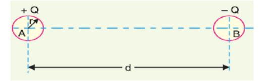
Fig 1.7: Single phase two wire transmission line
