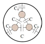
Fig 2.14- Cable Capacitance
