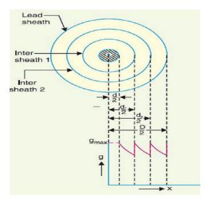
Fig 2.13- Intersheath grading
