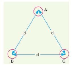
Fig 1.8 Three phase symmetrically spaced transmission line
