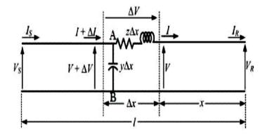
Fig.1.15: Modeling of long transmission line
