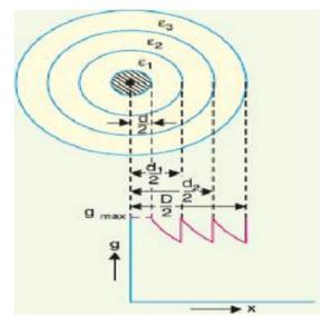
Fig 2.12- Capacitance grading
