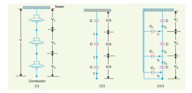
Fig 2.3- Suspension Insulator string
