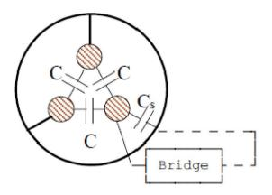
Fig 2.16-Capacitance Measurement
