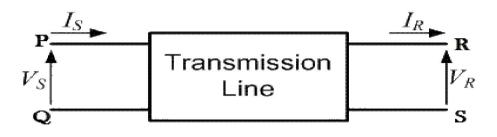
Fig 1.10: Representation of Two port network
