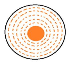
Fig.1.16: Current distribution in a conductor
