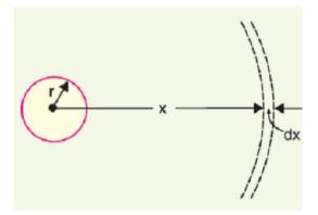
Fig 1.3: External flux linkage in a conductor
