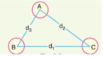
Fig 1.4 Three phase Overhead line
