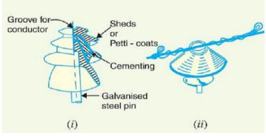
Fig 2.1- Pin Insulator
