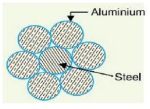
Fig 1.1:ACSR Conductor
