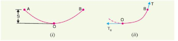
Fig 2.4- Sag in a transmission line
