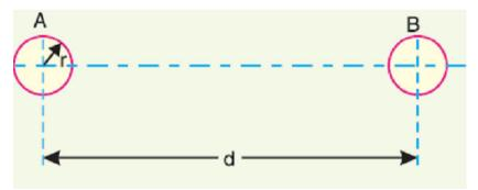
Fig 1.4: Single phase two wire transmission line
