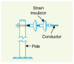
Fig 2.2- Strain Insulator
