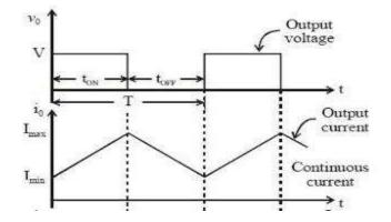
Figure: 3.4 current limit control waveforms
