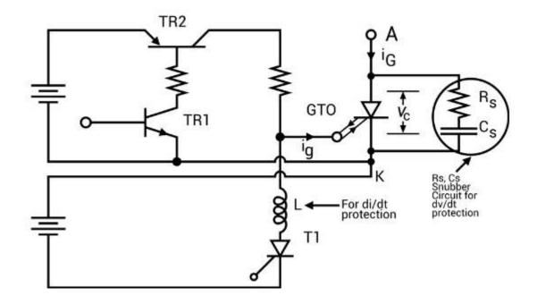
Figure: 1. 48. Gate Drive Circuit for GTO
