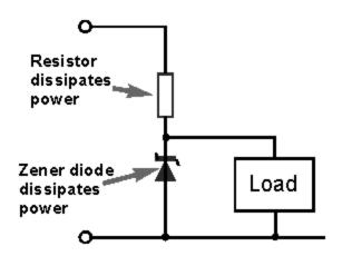
Figure: 3.19 Potential divider circuits
