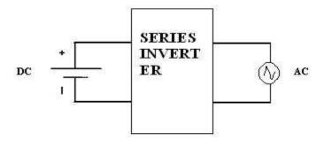
Figure: 5.11 Block diagram of series inverter
