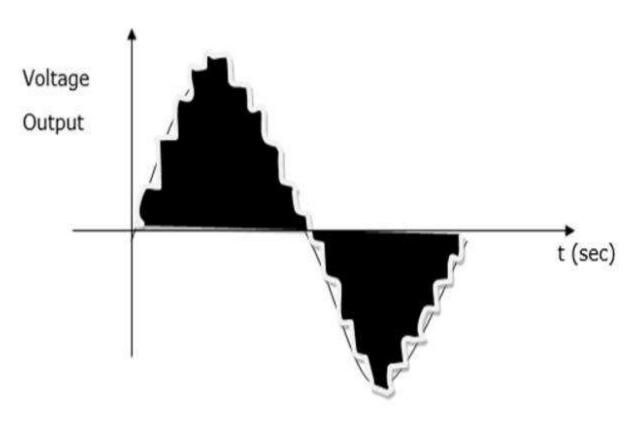
Figure: 5.31 Waveform of multiple PWM technique
