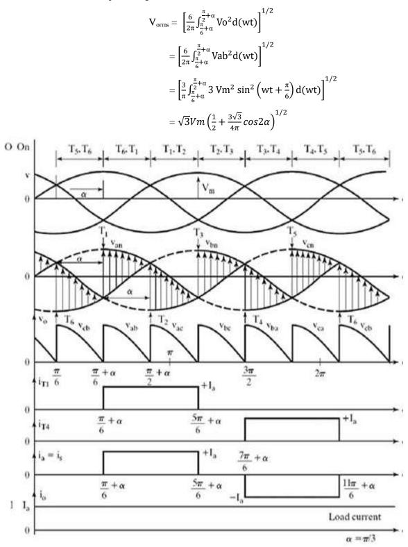
Figure: 2.21 Input and output waveforms of three phase fully controlled rectifier
