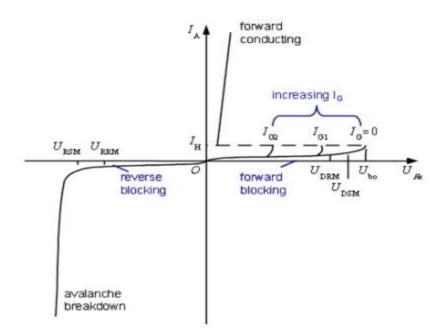
Figure: 1. 13. V - I characteristics of SCR
