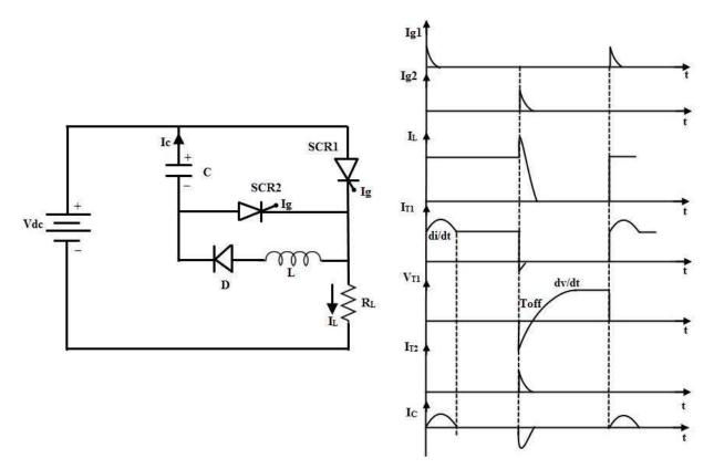
Figure: 1. 19. Class D Commutation circuit and waveforms
