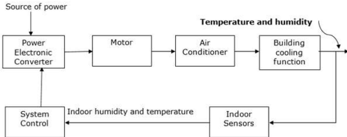
**Figure: 1.3. Block diagram of Air Conditioning System**
