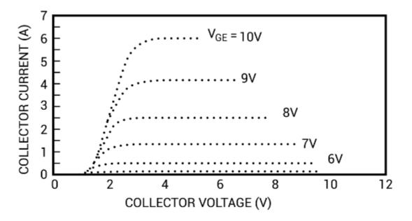
Figure: 1. 44. Forward characteristics of IGBT
