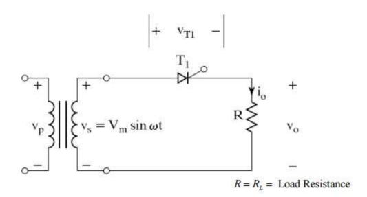
Figure: 2.2. Single phase half wave rectifier circuit
