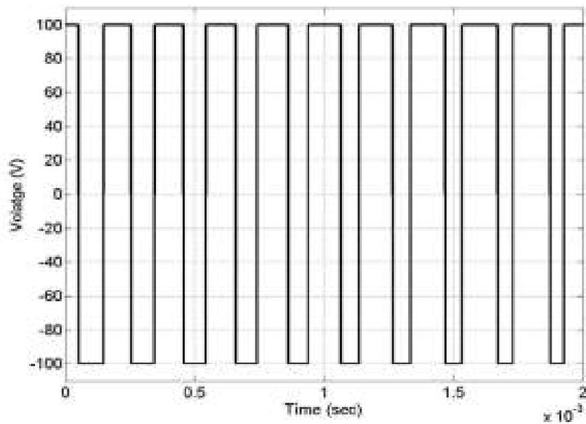
Figure: 5.34 Output voltage of the Half-Bridge inverter
