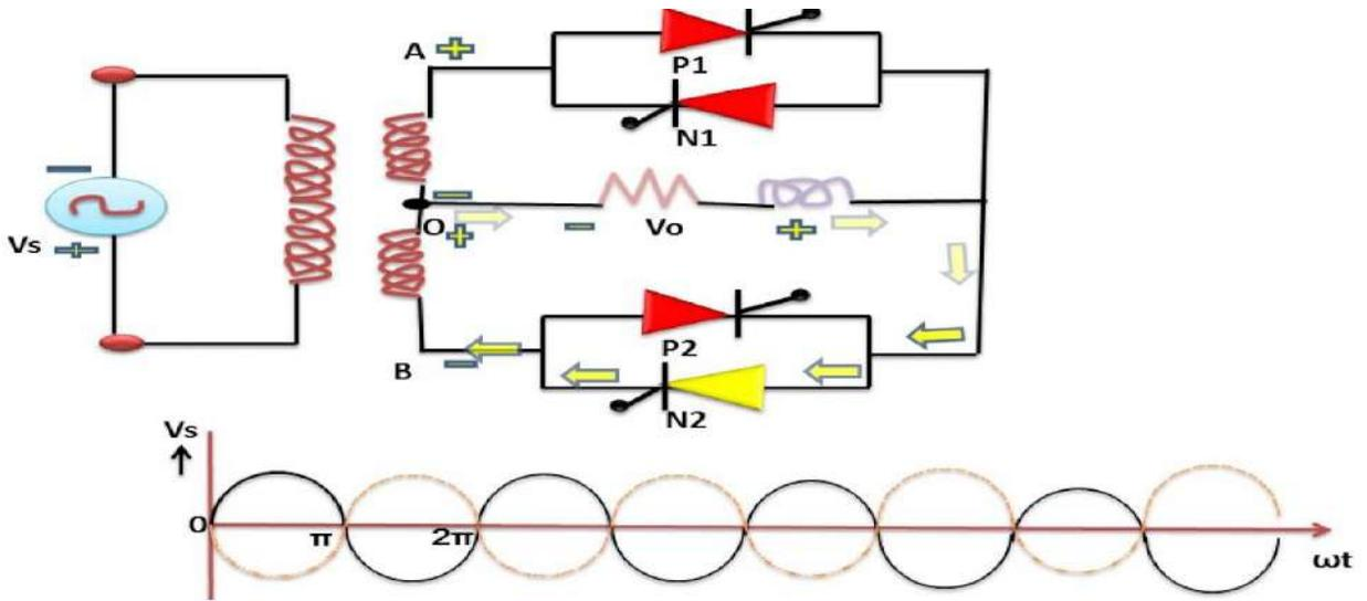
Figure 3.14 circuit diagram of midpoint cycloconverter
