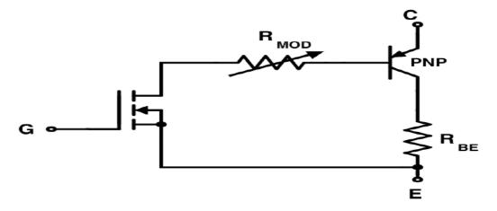
Figure: 1. 42. Simplified Equivalent diagram of IGBT
