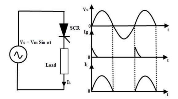
Figure: 1. 21. Natural Commutation circuit and waveforms
