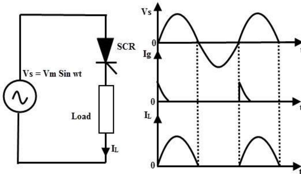
Figure: 1. 21. Natural Commutation circuit and waveforms
