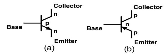
Figure: 1. 32. Symbol of transistor
