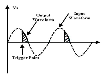
Figure: 1. 25. R Firing circuit waveforms of SCR
