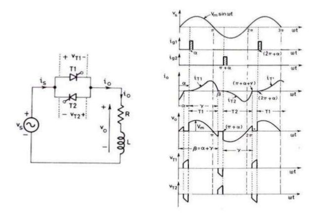
Figure: 3.3 Circuit diagram and output waveforms of AC voltage controller with RL load
