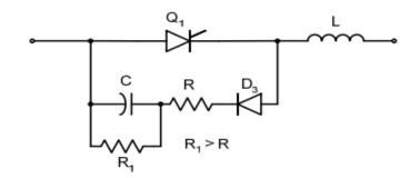
Figure: 1. 30. Reverse Polarized RC Snubber Circuit
