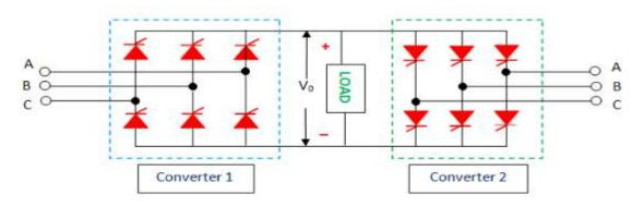
Figure: 2.33 Three phase dual converter
