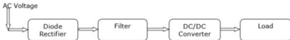
**Figure: 1.2. Block diagram of DC power supply**
