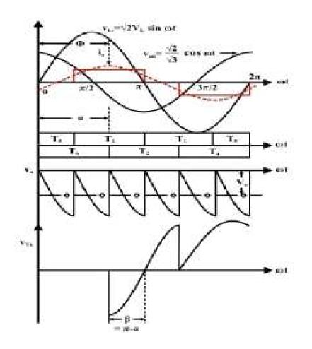
Figure: 2.24 Input and output waveforms of three phase fully controlled rectifier in inversion mode Effect of source inductance in three phase rectifiers
