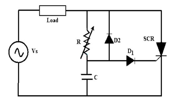
Figure: 1. 24. R Firing circuit for SCR
