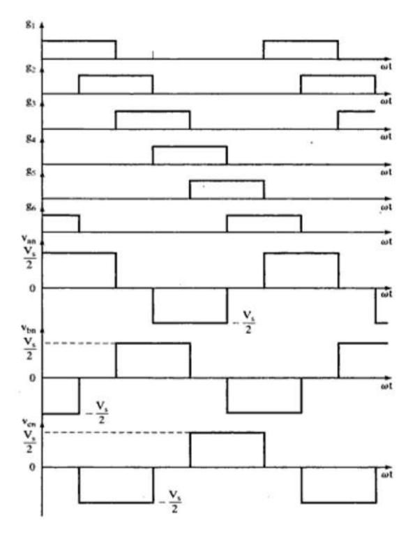
Figure: 5.26 Line and phase voltages of three phase bridge inverter
