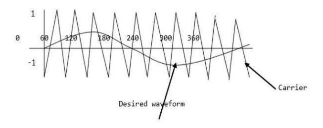
Figure: 5.28 Sinusoidal PWM waveform
