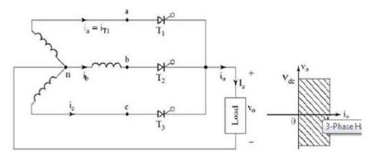
Figure: 2.16 circuit diagram three phase half wave rectifier
