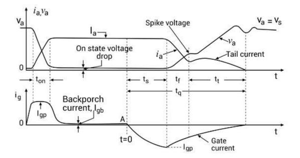
Figure: 1. 49. Switching characteristics for GTO
