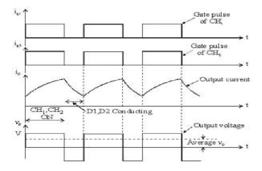
Figure: 3.17 Output voltage and current waveforms of type D chopper
