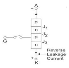
Figure: 1.7. Reverse blocking mode of SCR
