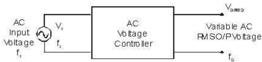
Figure: 3.1 Block diagram of AC voltage controller
