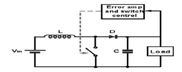
Figure: 3.24 circuit diagram of Boost regulator
