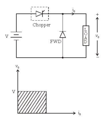
Figure: 3.10 circuit diagram and quadrant operation of Type A chopper
