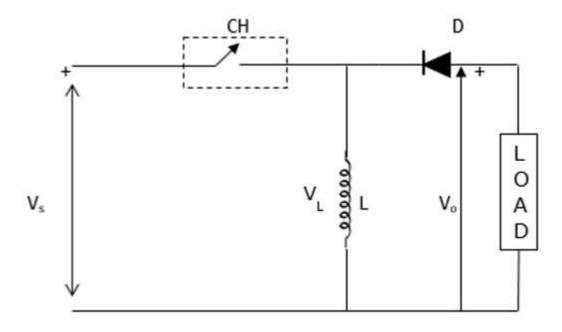
Figure: 3.9 circuit diagram of step up chopper
