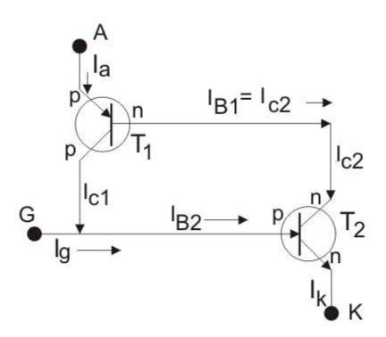
Figure: 1. 12. Two transistors connection of SCR
