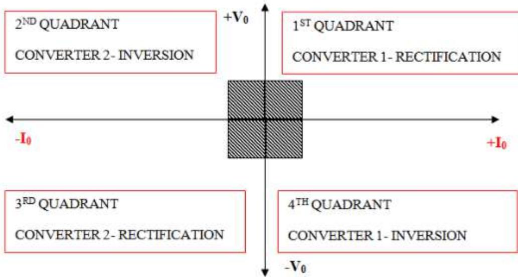
Figure: 2.29 Four quadrant operations of dual converter
