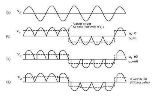
Figure 3.13 Input and output waveforms of cycloconverter
