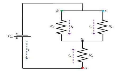
Figure: 5.20 Current flow in Mode 2 operation
