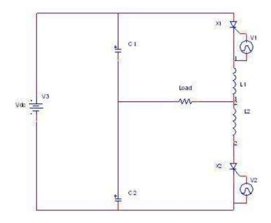
Figure: 5.12 Circuit diagram of series inverter
