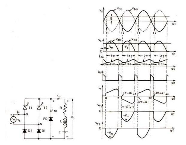
Figure: 2.6 single phase half controlled converter with RLE load and freewheeling diode
