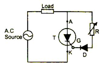
Figure: 1. 14. Resistance triggering circuit of SCR
