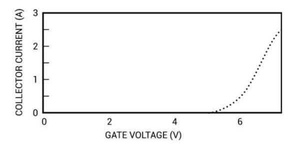
Figure: 1.45. Transfer characteristics of IGBT
