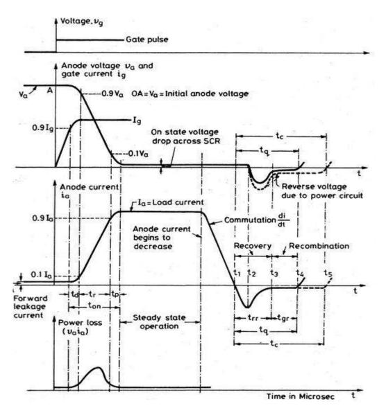
Figure: 1. 22. Dynamic characteristics of SCR
