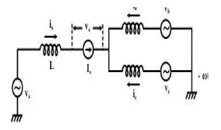
Figure: 2.27 Equivalent circuit of waveforms with source inductance
