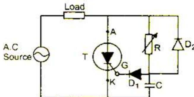
**Figure: 1. 15. Resistance Capacitance triggering circuit of SCR**
