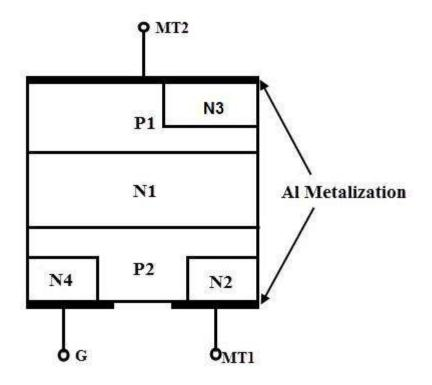
Figure: 3.5 construction of TRIAC
