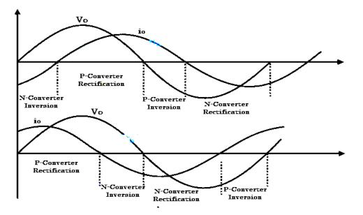
Figure 3.17 cycloconverter waveforms
