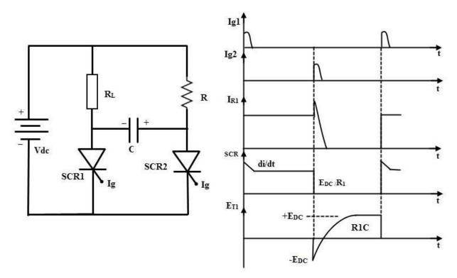
Figure: 1. 18. Class C Commutation circuit and waveforms
