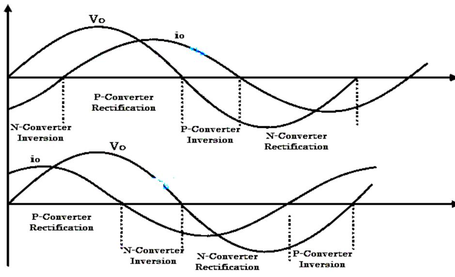
Figure 3.17 cycloconverter waveforms
