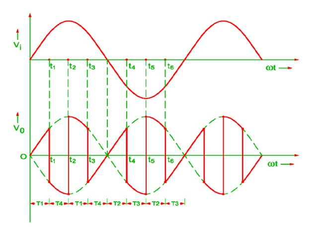
Figure 3.15 Input and output waveforms of midpoint cycloconverter
