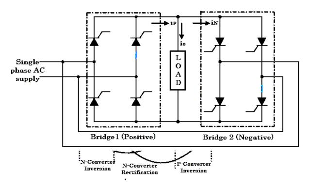
Figure 3.18 Circuit diagram of bridge type cycloconverter
