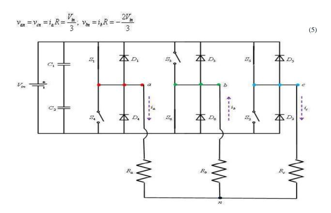
Figure: 5.17 Mode 1 operation of three phase bridge inverter with star connected load
