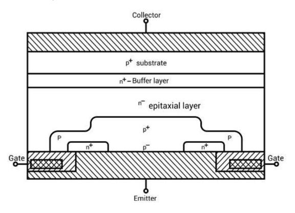
Figure: 1. 40. Cross -sectional structural diagram of IGBT
