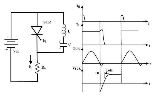
Figure: 1. 17. Class B Commutation circuit and waveforms
