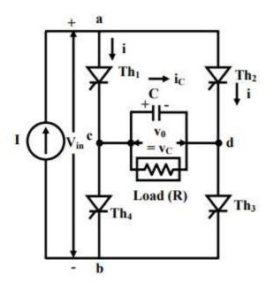
Figure: 5.39 Circuit diagram of load commutated CSI
