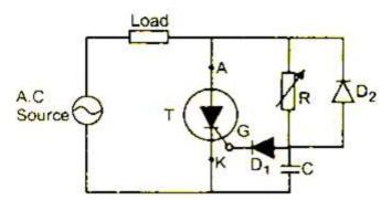
Figure: 1. 15. Resistance Capacitance triggering circuit of SCR
