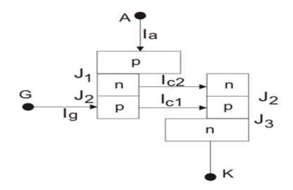
Figure: 1. 11. Two transistor structure of SCR
