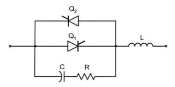
Figure: 1. 31. An un-polarized snubber circuit
