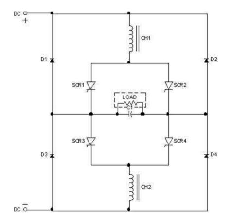
Figure: 5.14 Circuit diagram of parallel commutated inverter
