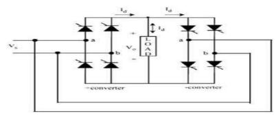
Figure 3.12 circuit diagram of cycloconverter
