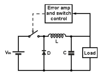
Figure: 3.20 circuit diagram of Buck regulator
