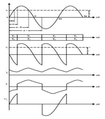
Figure: 2.10 single phase full converter circuit with RL load input and output waveforms
