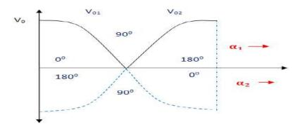
Figure: 2.32 output voltage variation with firing angle
