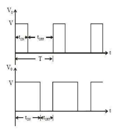
Figure: 3.2 pulse width modulation waveforms
