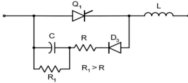
**Figure: 1. 30. Reverse Polarized RC Snubber Circuit**
