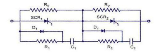
Figure: 1. 27. Series connection of SCRs
