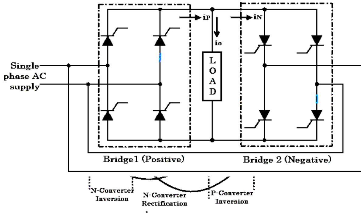
Figure 3.18 Circuit diagram of bridge type cycloconverter
