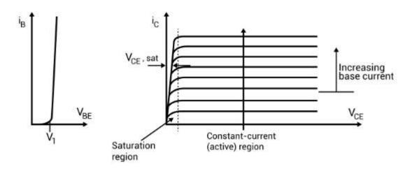
Figure: 1. 34. Input and output characteristics of BJT
