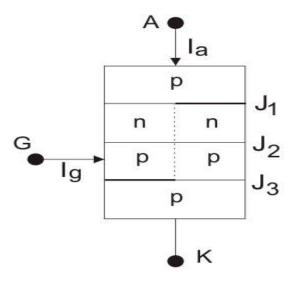
Figure: 1.10. Two transistor structure of SCR
