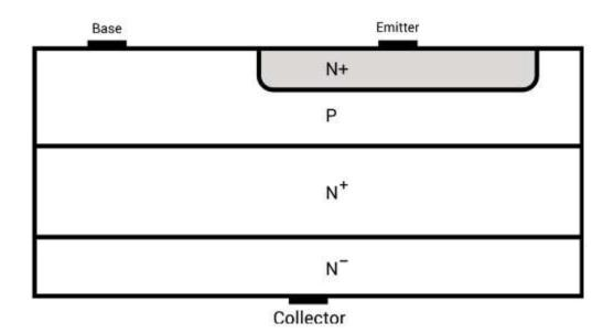
Figure: 1. 33. Structure of transistor
