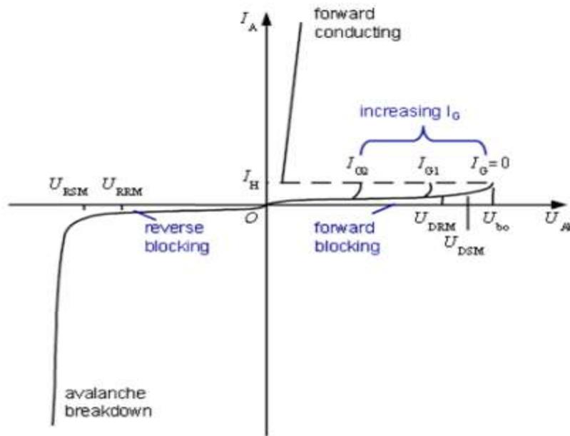
**Figure: 1. 13. V - I characteristics of SCR**
