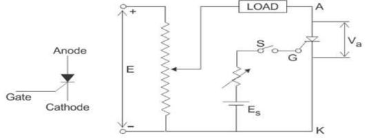
Figure: 1.6. Circuit diagram for characteristics of SCR
