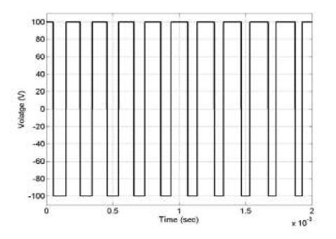
Figure: 5.34 Output voltage of the Half-Bridge inverter
