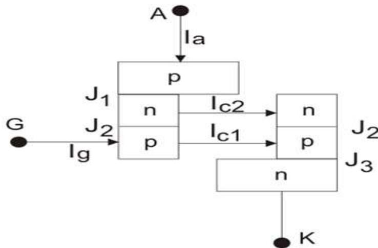
Figure: 1. 11. Two transistor structure of SCR
