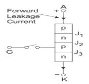
Figure: 1.9. Forward connection of SCR
