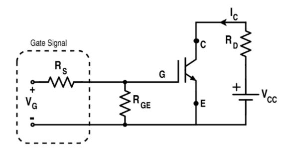
Figure: 43. Equivalent diagram of IGBT
