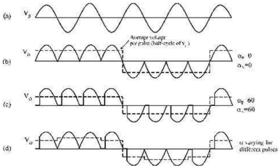
**Figure 3.13 Input and output waveforms of cycloconverter**
