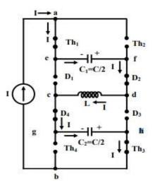
Figure: 5.37 Mode I operation of CSI
