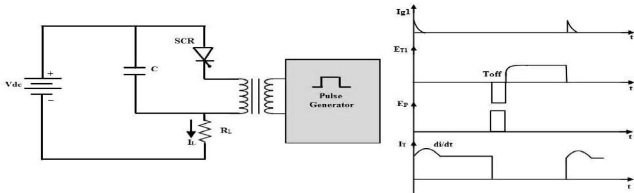
Figure: 1. 20. Class E Commutation circuit and waveforms
