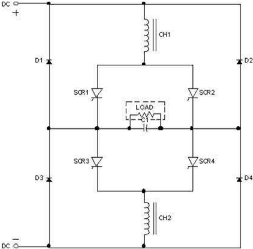
**Figure: 5.14** Circuit diagram of parallel commutated inverter
