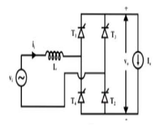
Figure: 2.13 single phase full converter circuit with source inductance
