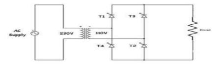
Figure: 2.7 single phase full converter circuit with R load
