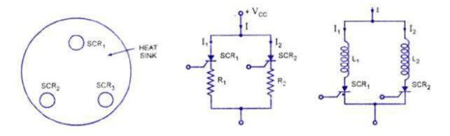
Figure: 1. 28. Parallel connection of SCRs
