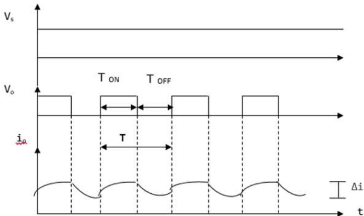
Figure: 3.6 Input and output waveforms
