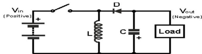
Figure: 3.27 circuit diagram of buck boost regulator
