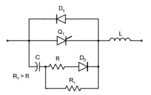
Figure: 1. 29. Forward-Polarized RC Snubber Circuit
