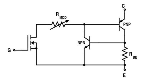
Figure: 1. 41. Equivalent diagram of IGBT
