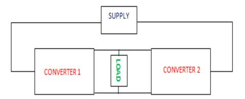
Figure: 2.28 Block diagram of dual converter
