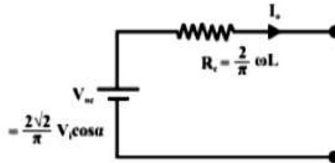
**Figure: 2.15** Equivalent circuit of the given equation
