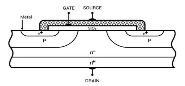
Figure: 1. 36. Structure of MOSFET
