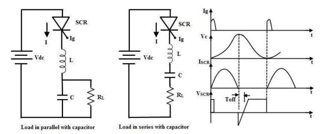
Figure: 1. 16. Class A Commutation circuit and waveforms
