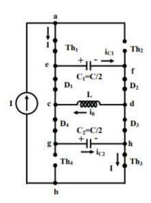
Figure: 5.38 Mode II operation of CSI
