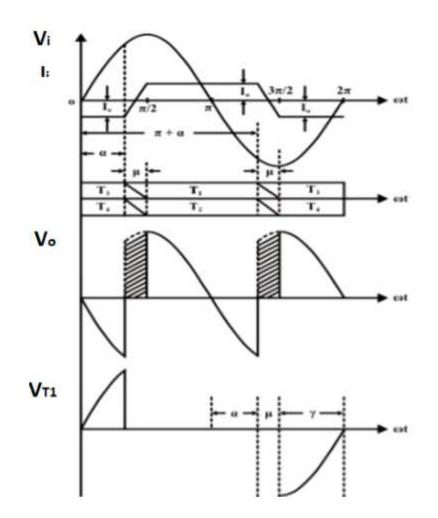
Figure: 2.14 single phase full converter output waveforms with source inductance
