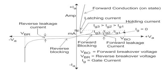
Figure: 1.8. V- I characteristics of SCR
