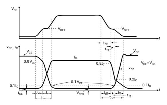
Figure: 1. 46. Dynamic characteristics of IGBT
