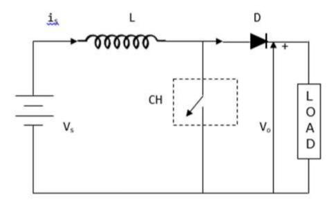
Figure: 3.7 circuit diagram of step up chopper
