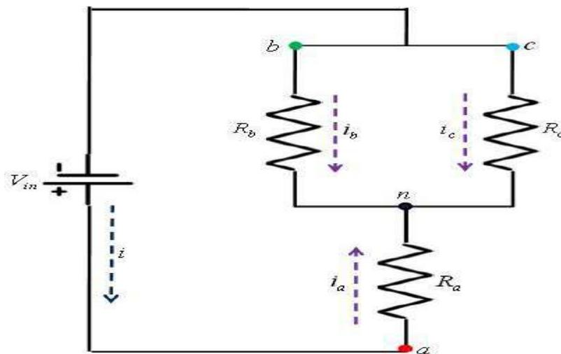
Figure: 5.20 Current flow in Mode 2 operation
