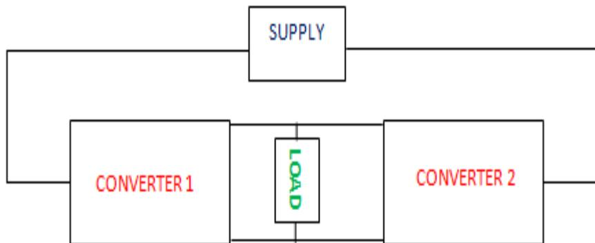
**Figure: 2.28 Block diagram of dual converter**
