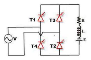
Figure: 2.11 single phase full converter circuit with RLE load
