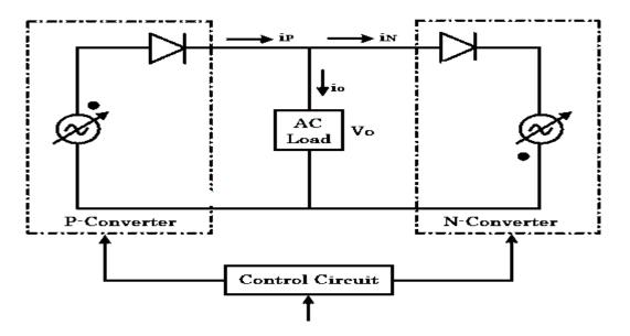
Figure 3.16 Block diagram of bridge type cycloconverter
