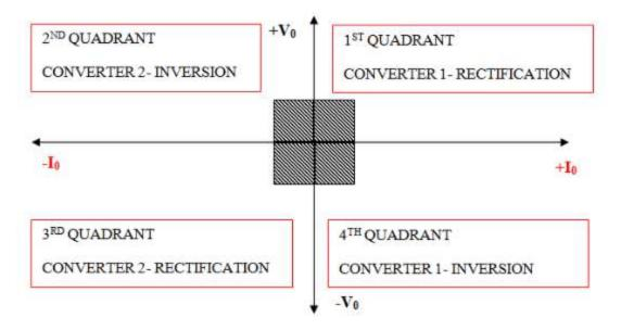
Figure: 2.29 Four quadrant operations of dual converter
