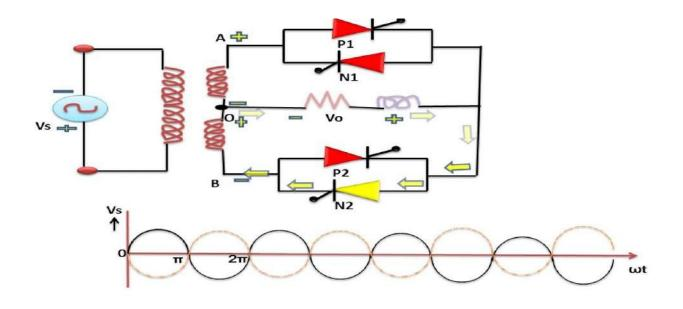
Figure 3.14 circuit diagram of midpoint cycloconverter
