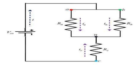
Figure: 5.23 Current flow in Mode 3 operation
