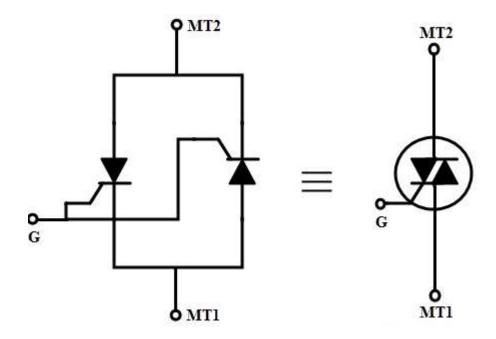
Figure: 3.4 Two thyristor analogy and circuit symbol of TRIAC
