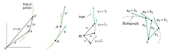
**Hodograph:** A curve the radius vector of which represents in magnitude and direction the velocity of a moving object.
