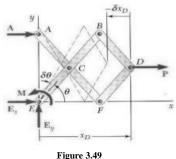
**Problem No 2:** Using principle virtual work find the value of the angle  $\theta$  defining the configuration of equilibrium of the system shown in figure below The ball D and E can slide freely along the bars AC and BC, but the string DE connecting the balls is inextensible.
