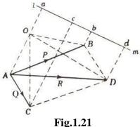
**Proof**: The moments of both forces P and Q with respect to centre 'O' as shown in figure. the moment of resultant force R. Joining OA and extended the line OA, draw the perpendicular *l-m* to the line OA. Joining the perpendiculars Aa, Bb, Cc and Dd
