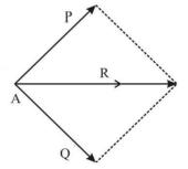
**Fig.1.3. Principle of superposition**
