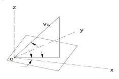
(16) An aircraft takes off at A and climbs at a steady angle with slope of 1 to 2 in the vertical y-z plane at a constant speed v = 400 km/h. The aircraft is tracked by radar at O. For the position B, determine the value of  $R\theta$ , and  $\phi$ .
