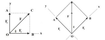
**Fig.1.10 Rectangular Force Components**
